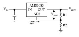
$$V_{OUT} = V_{REF} (1 + R2/R1) + I_{ADJ}R2$$
