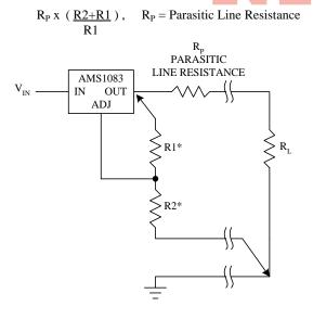
\*CONNECT R1 TO CASE CONNECT R2 TO LOAD
