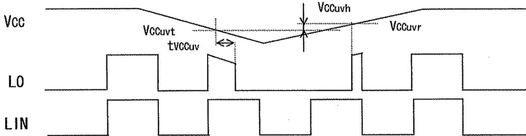
When Vcc Supply Voltage keeps lower UV Trip Voltage( $V_{CCUVt} = V_{CCUVr} - V_{CCUVh}$ ) for Vcc Supply UV Filter Time, output signal becomes "L". And then, when Vcc Supply Voltage is higher than UV Reset Voltage, input signal (LIN) is L; output signal HO becomes "H".
