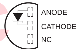
LP (TO-92/TO-226) PACKAGE (TOP VIEW)
