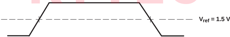
Figure 7-2. Input and Output Voltage Reference Levels for AC Timing Measurements
